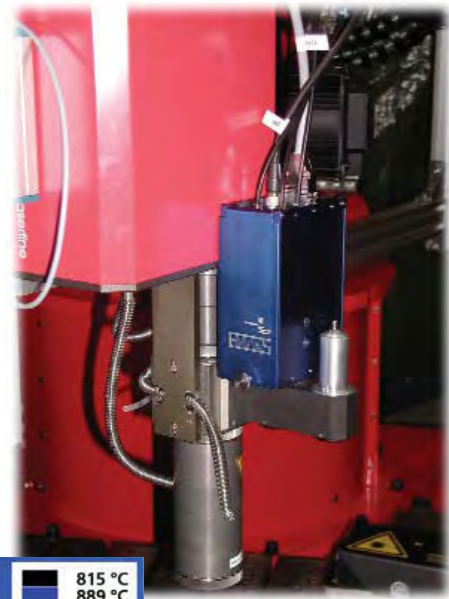
E-Maqs Camera on Diode Laser
