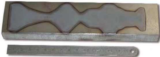
Laser Hardening with Variable Track Width
